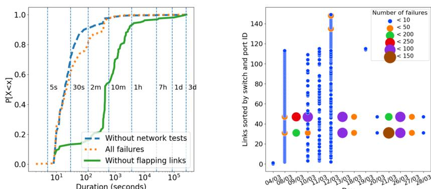
(a) Cumulative distribution of failure duration, which includes all failures, failures observed excluding test periods and treats flapping links as a single failure. (b) Distribution of failures for each link and day of March 2024. The links on the y axis are sorted by switch and port ID.
