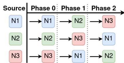
Figure 2. The all-to-all exchange between 3 nodes divided into 3 phases.
