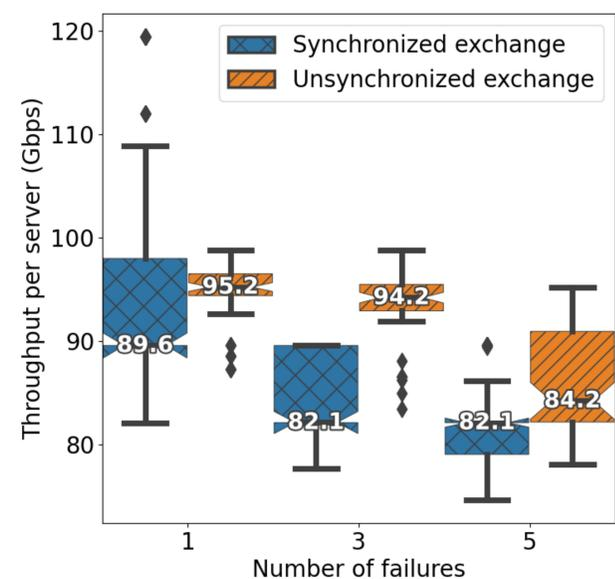
Figure 5. Synchronized and unsynchronized all-to-all exchange throughput as a function of the number of failures. Failure scenarios are randomly generated 10 times with 1, 3 or 5 simultaneous failures on the Event Builder network. The boxplots represent the minimum, 25th percentile, median, 75th percentile, and maximum values. Outliers are also depicted.
