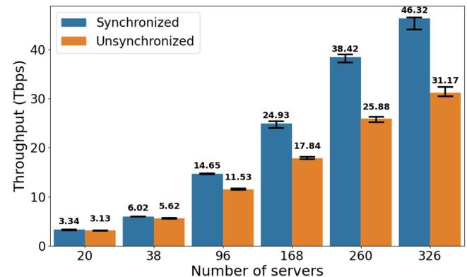
Figure 4. Scalability of the synchronized and unsynchronized all-to-all applications. The error bars represent the minimum, mean and maximum values.
